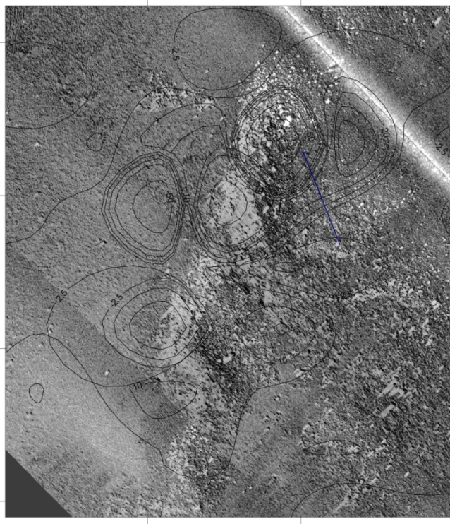
Fig. 5.7. Example of an object (torpedo weighing approximately 1.5 tons) on the sea bottom combined with the values of magnetic field anomalies
